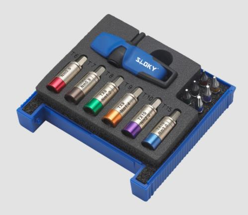
A multiset kit of the World's Smallest Torque Screwdriver, with a specially customized universal handle with 6 torque adapters (0.6 ~ 6Nm) and bits of Torx.
